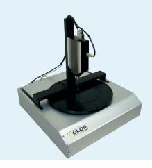
FR-Scanner scans the wafers by rotating the wafer and by moving it linearly (Polar Coordinates) with unparalleled speed and accuracy in both radius and angle. This way, accurate reflectance data with high repeatability are recorded, making FR-Scanner the ideal tool for at-line and on-line characterization of coatings on wafers or other substrates at processing facilities.
