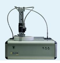
FR-pRo is assembled by user selected modules. The Core Unit accommodate the light source, the spectrometer (for any spectral regime in the 200 nm - 2500 nm range) and the control & communication electronics. Then, there is a wide range of accessories, such as:
