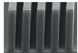
5 \mu\text{m} dense line/space in 25 \mu\text{m} film
